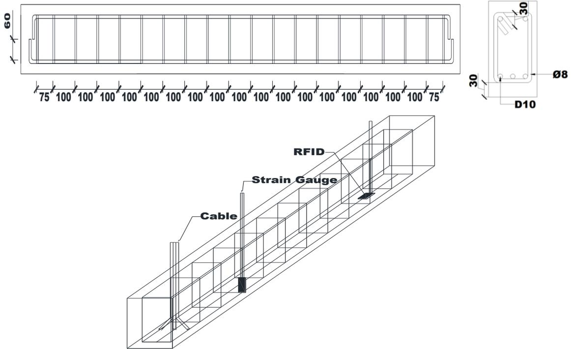
Figure 2. Details of beam geometry and test setup
