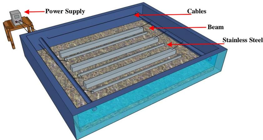
**Figure 4. Setup of galvanostatic method**
