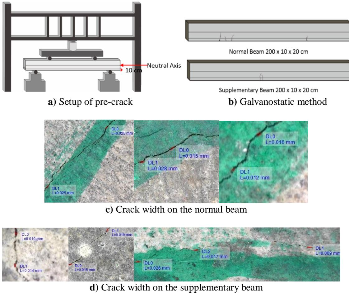
**Figure 3. Precrack test of beams**
