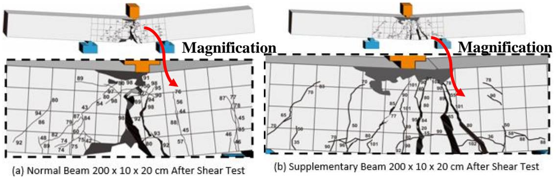
**Figure 8. Crack pattern after shear test**
