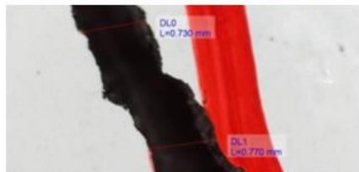
(b) Supplementary Beam Crack Width
