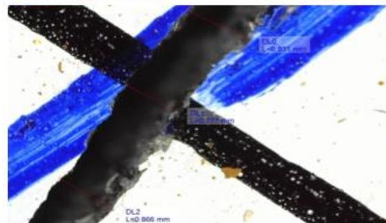
(a) Normal Beam Crack Width
