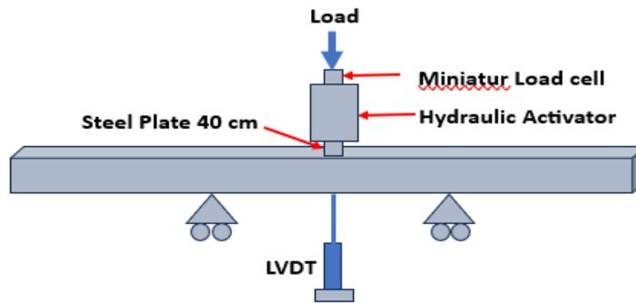
Figure 6. Setup shear test
