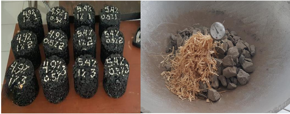
Figure 5. OGFC test specimen with bamboo fiber modification
