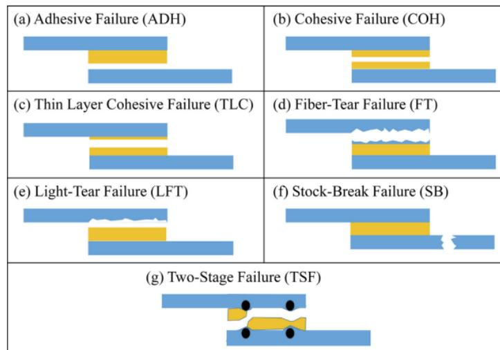
**Figure 1. Adhesive Joint Failure Modes [13]**
