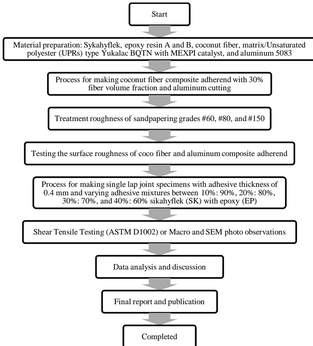
**Figure 3. Research Flow Diagram**
