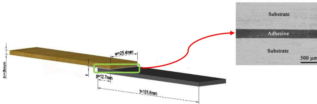
**Figure 2. Single Lap Joint Type Connection**
