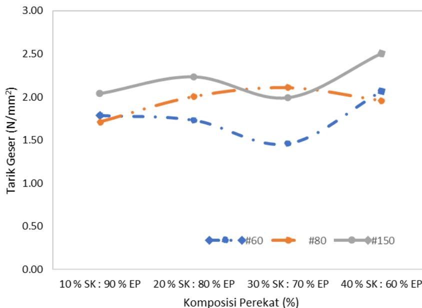
**Figure 6. Shear Tensile Test Results of Single Lap Joint Aluminum-Coco Fiber Composite**
