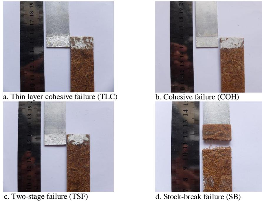
**Figure 7. Failure Modes in Aluminum-Composite Coco Fiber Joints**
