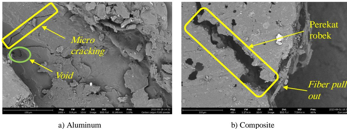
Figure 9. SEM Morphology Results of Mixed Adhesive
