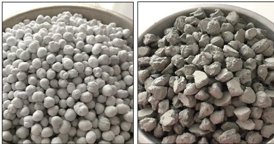
Figure 1. ALWA before coated and after mortar coated
